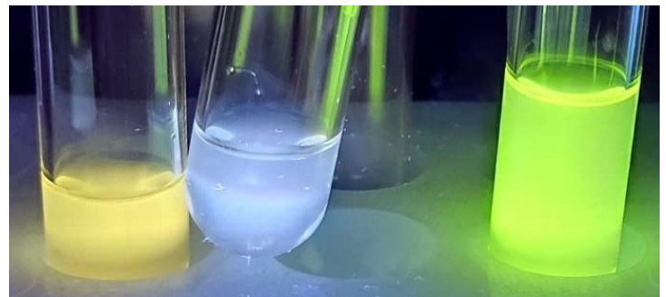
Yellow and blue luminescent colloidal solutions of carbon nanodots
